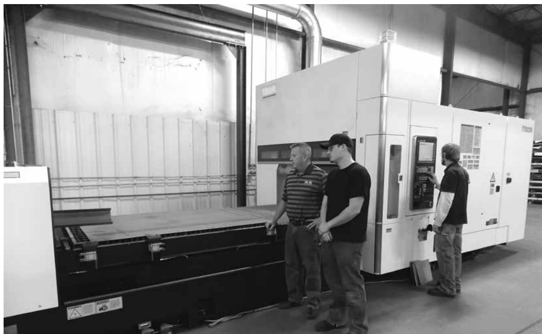
Above: Van-Am's Mazak 4,000-watt 5-axis laser cutting system can handle 2D & 3D work.
